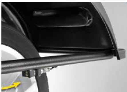
Sonar for automatic measurement of the wheel width. (Sirion Pro/S)
